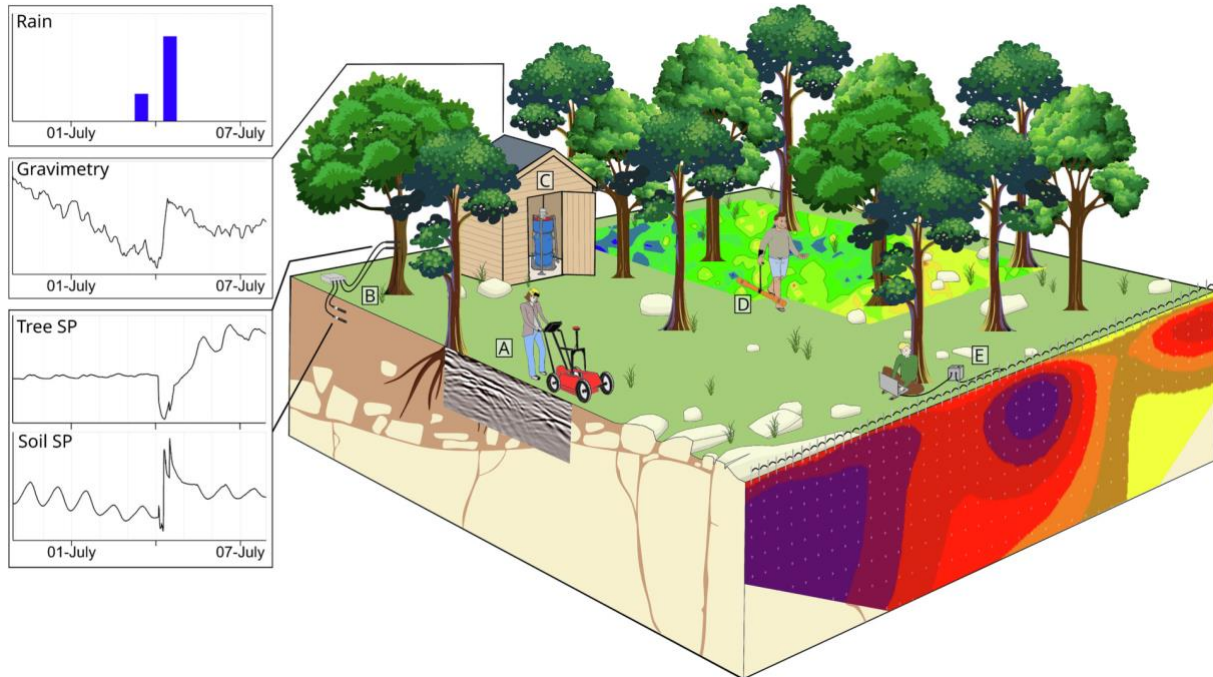
Figure 3: Field implementation of geophysical techniques discussed in Loiseau et al. (2023). The label (E) locate the electrical resistivity tomography (ERT) that can be used to characterize the spatial heterogeneity of subsurface properties around the tree-root systems and possibly monitor the water dynamics.
